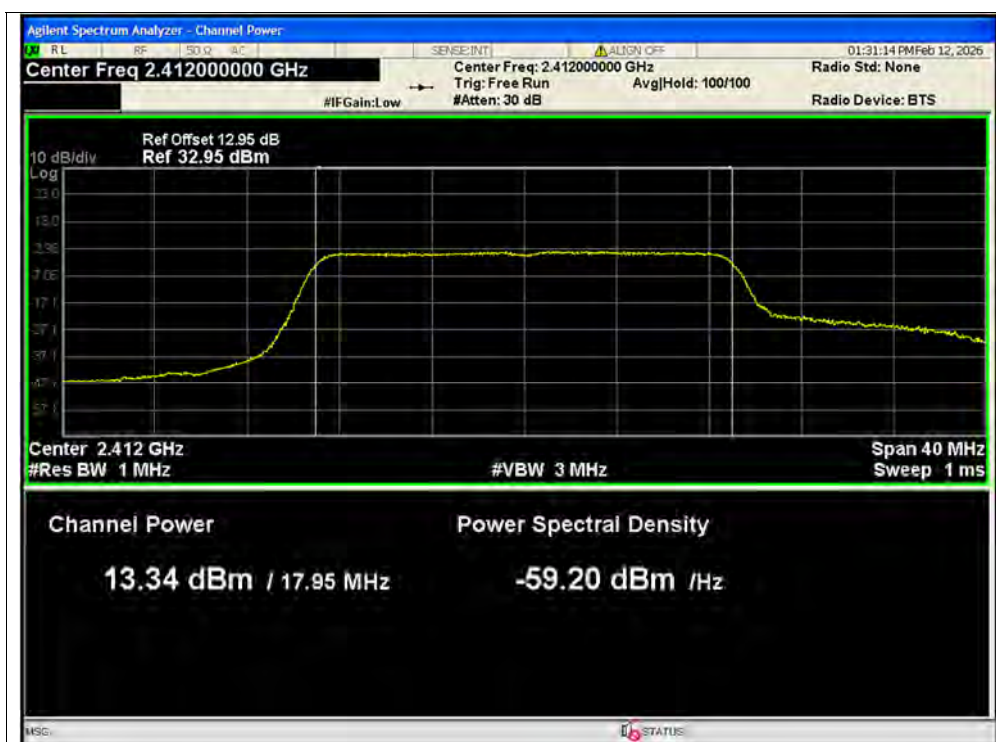
Average Power NVNT n20 2412MHz Ant1 MIMO
