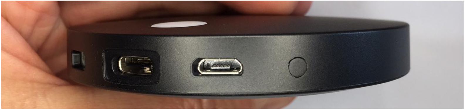
Inlet ports (USB-C, Micro USB), Kensington slot and reset button
