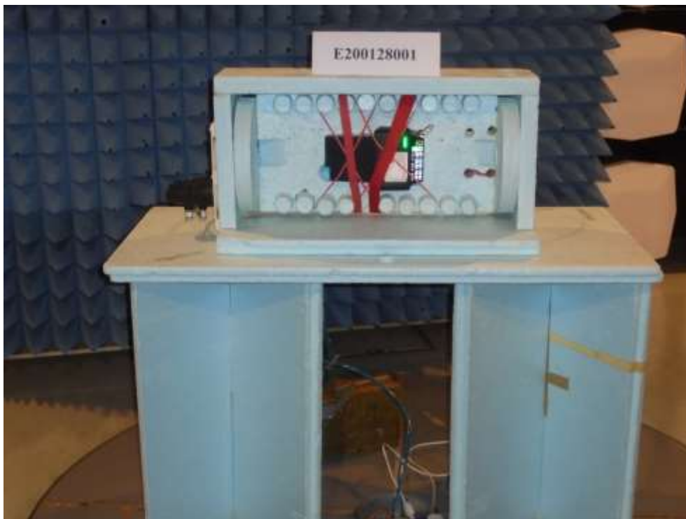
Test setup in semi anechoic chamber, worst case position, long shot view
