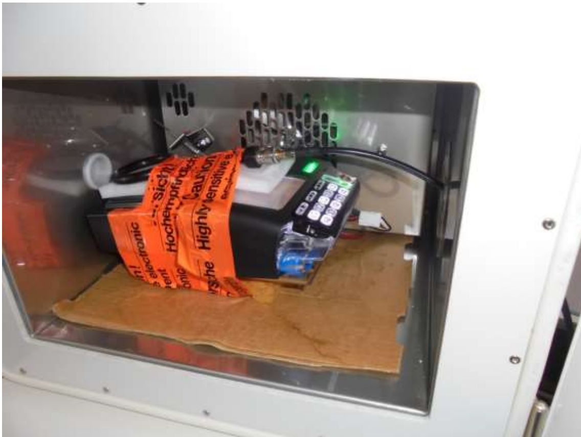
Test setup in radio lab, EUT inside climatic chamber
