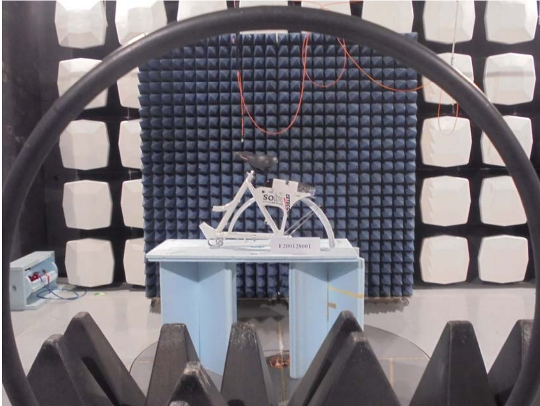
Test set-up vertical, tests < 30MHz
