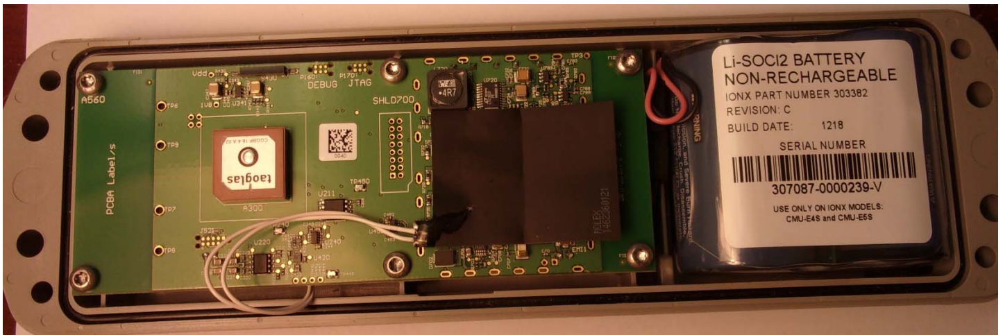
Model CMU-E5S, Internal Configuration
