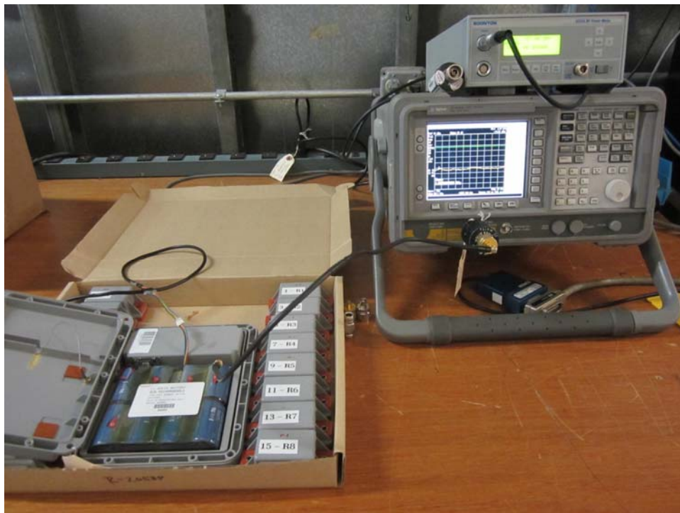
20 dB Bandwidth Test Setup
