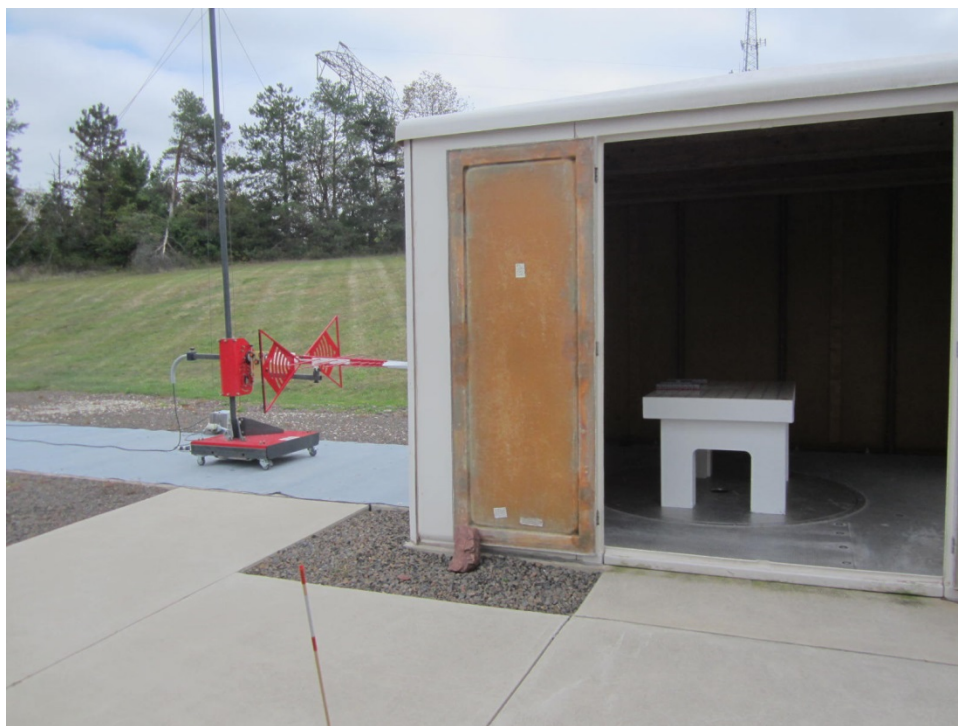
Field Strength of Spurious Emissions, Horizontal Antenna Polarization Below 1 GHz
