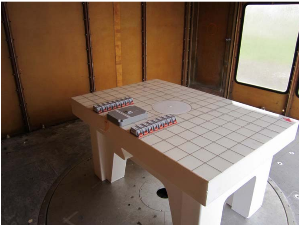
Field Strength of Spurious Emissions, Test Setup
