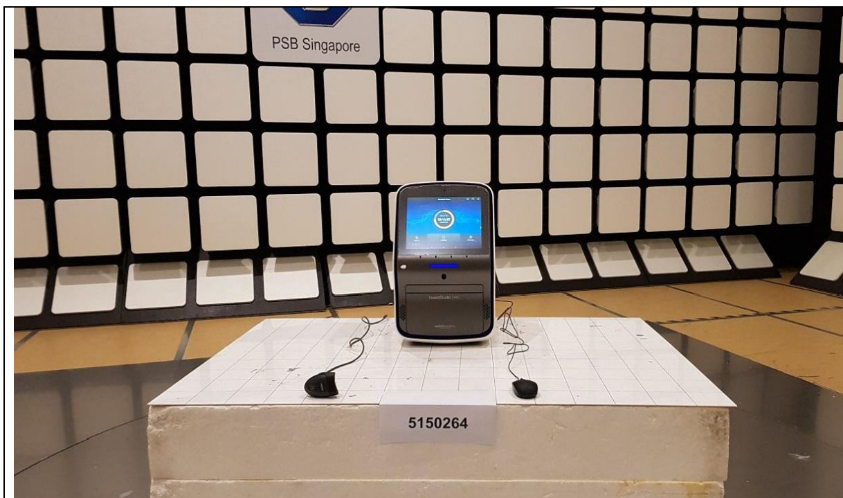
Radiated Emissions Test Setup (Front View)
