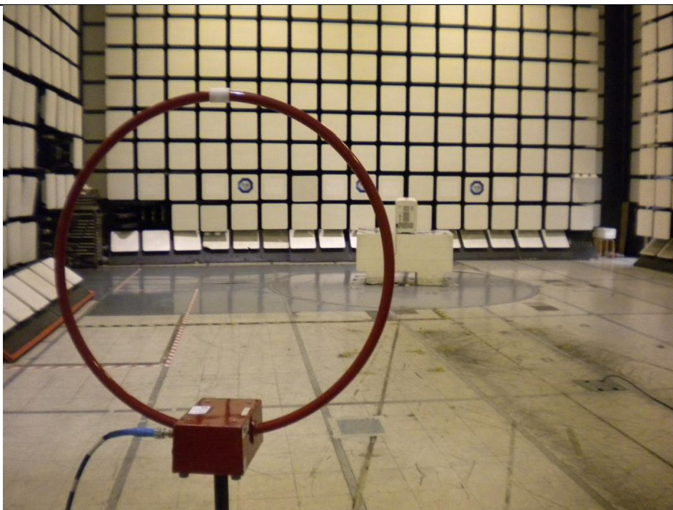
Radiated Emissions Test Setup (Front View)
