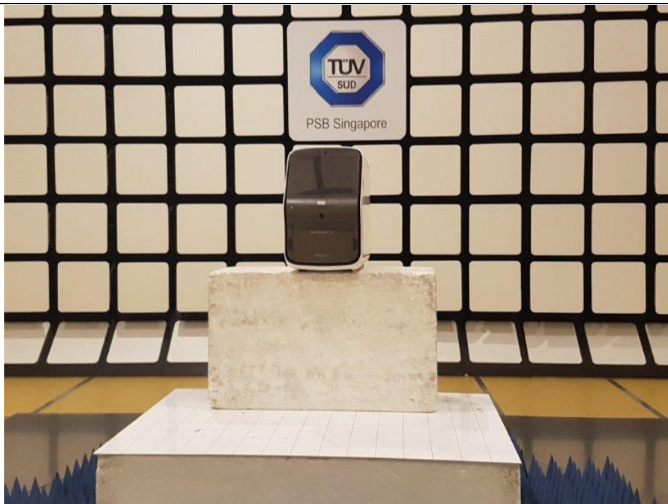
Radiated Emissions Test Setup (Front View)
