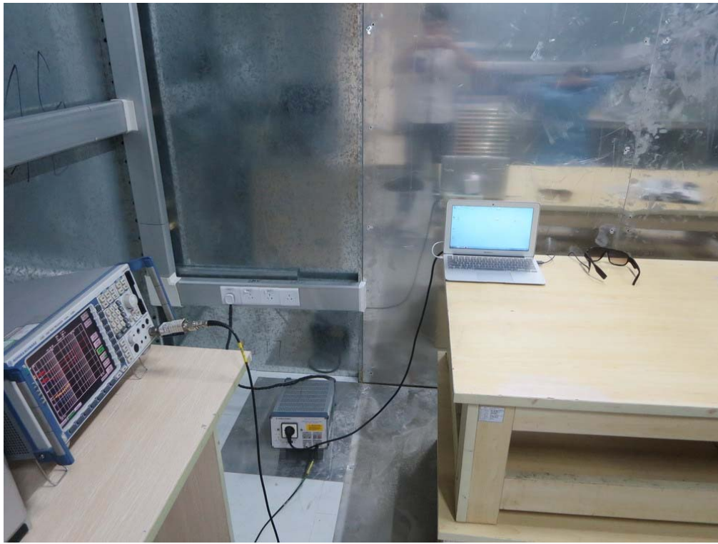
FCC RADIATED EMISSION TEST SETUP
