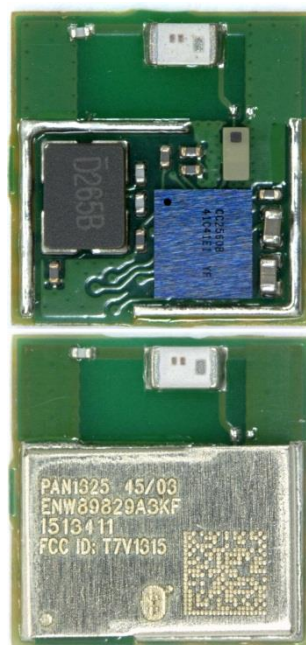
EUT (PAN 1325 - ENW89829A3KF) with and without shielding
