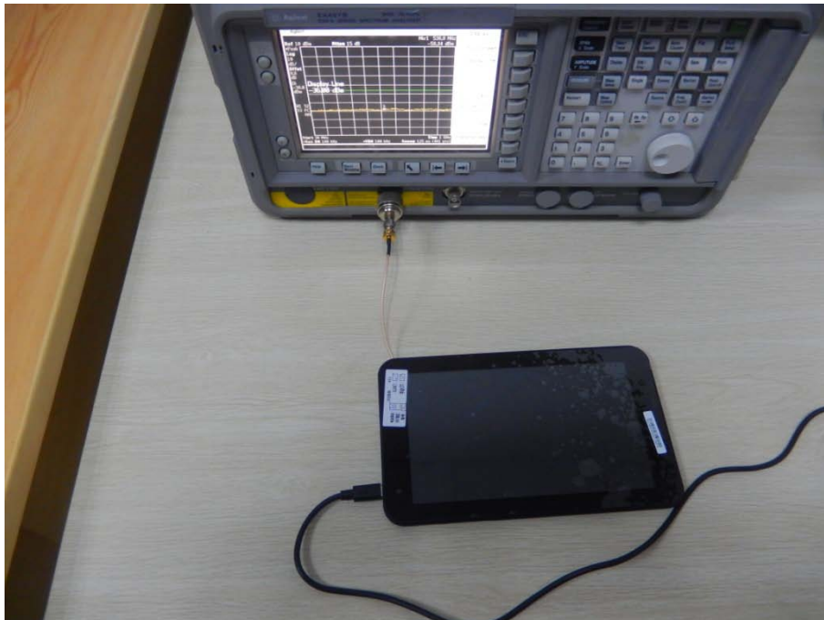
DSS&DTS RF conduction test photos
