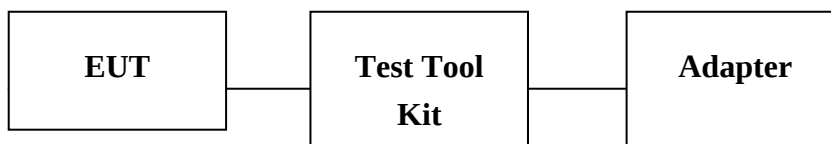
Fig. 2-2 AC Power Line Conducted Emission Configuration
