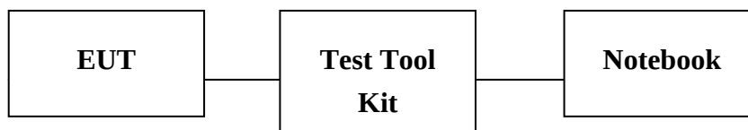
Fig. 2-2 Conducted Emission Configuration (Antenna Port)
