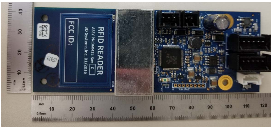
Top view – with EMI shield
