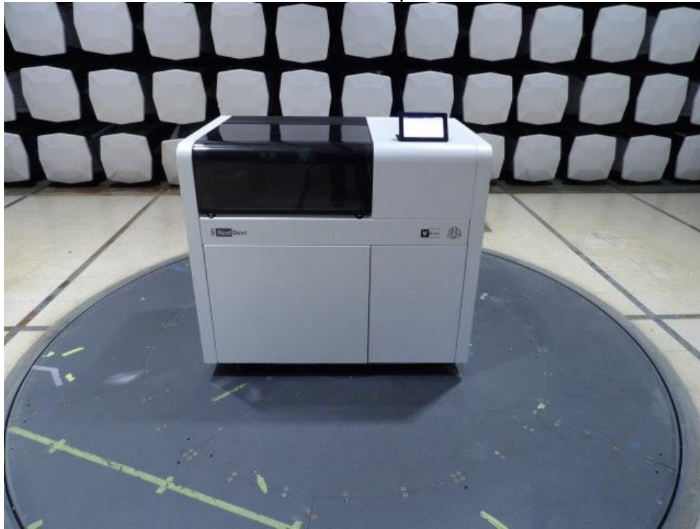
Radiated – Fundamental and Spurious below 30 MHz
