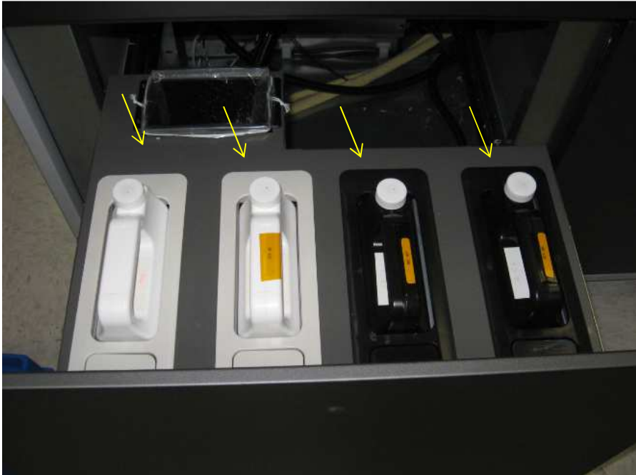
Material Distribution Module (MDM) with material bottles installed: Antenna locations are shown using arrows
