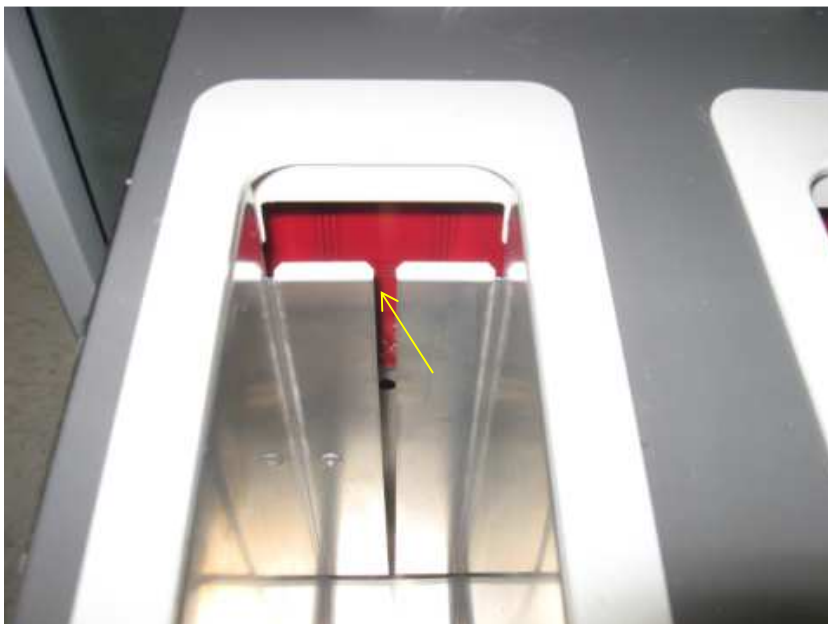
Material Distribution Module (MDM) with material bottles removed: Close-up view of antenna locations
