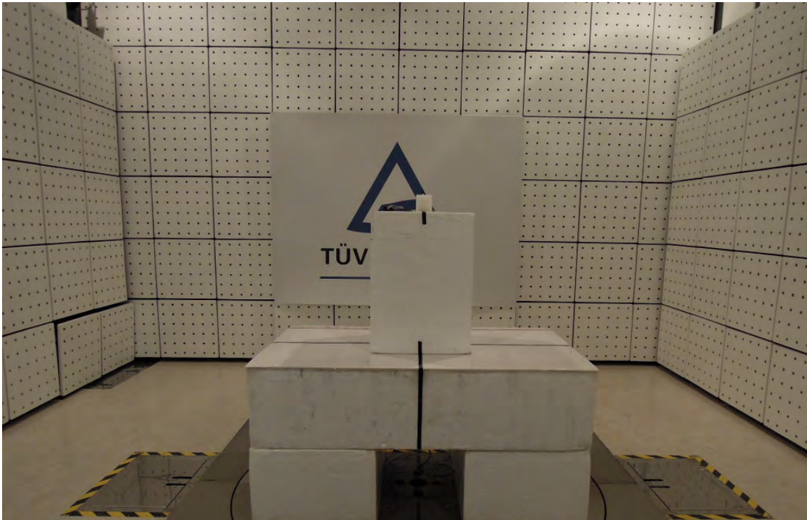
Photograph 20: Set-up for Spurious Emissions (Back View)- ACC-RN-SMA-S-DS -ANT
