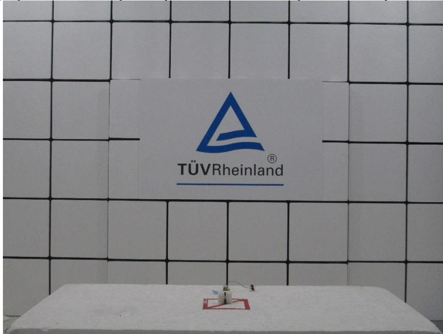
Photograph 2: Test Setup for Spurious Emissions (Front View 2)
