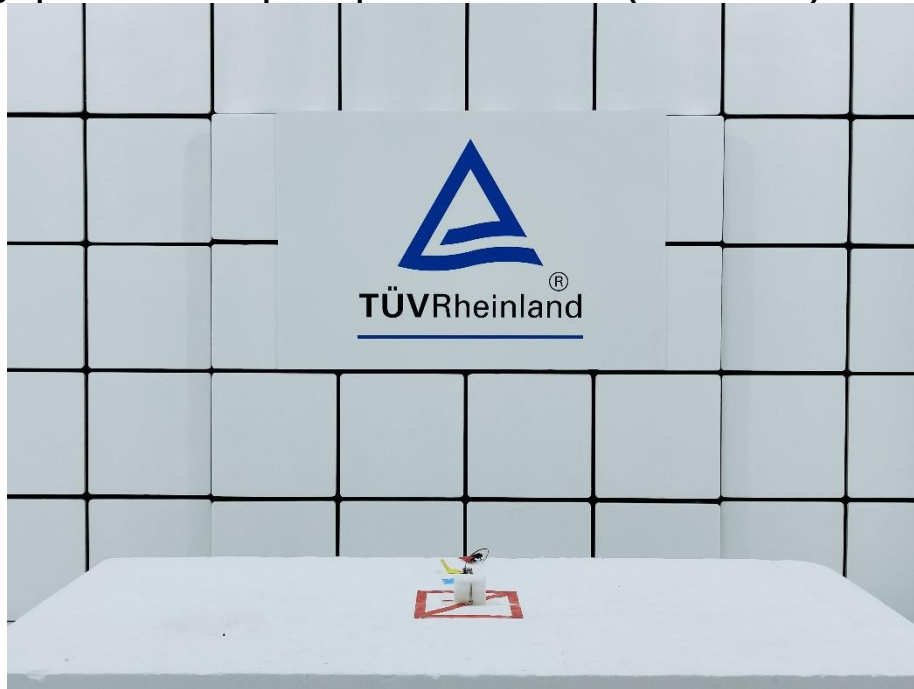
Photograph 14: Test Setup for Spurious Emissions (Front View 2)
