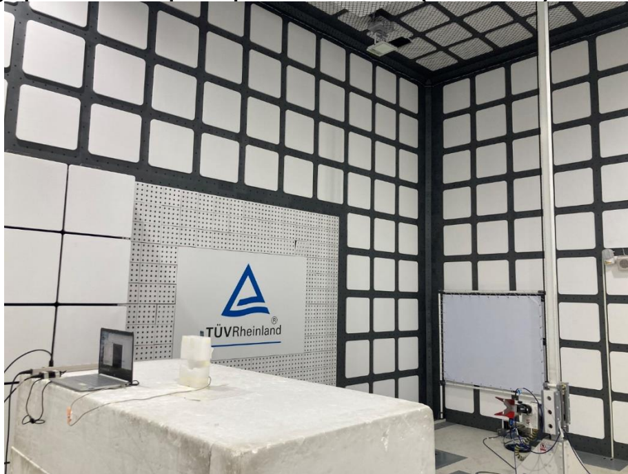
Photograph 6: Test Setup for Spurious Emissions (Back View 4)
