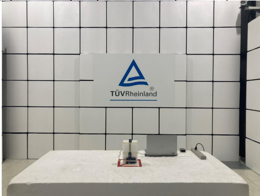
Photograph 10: Test Setup for Spurious Emissions (Front View 2)
