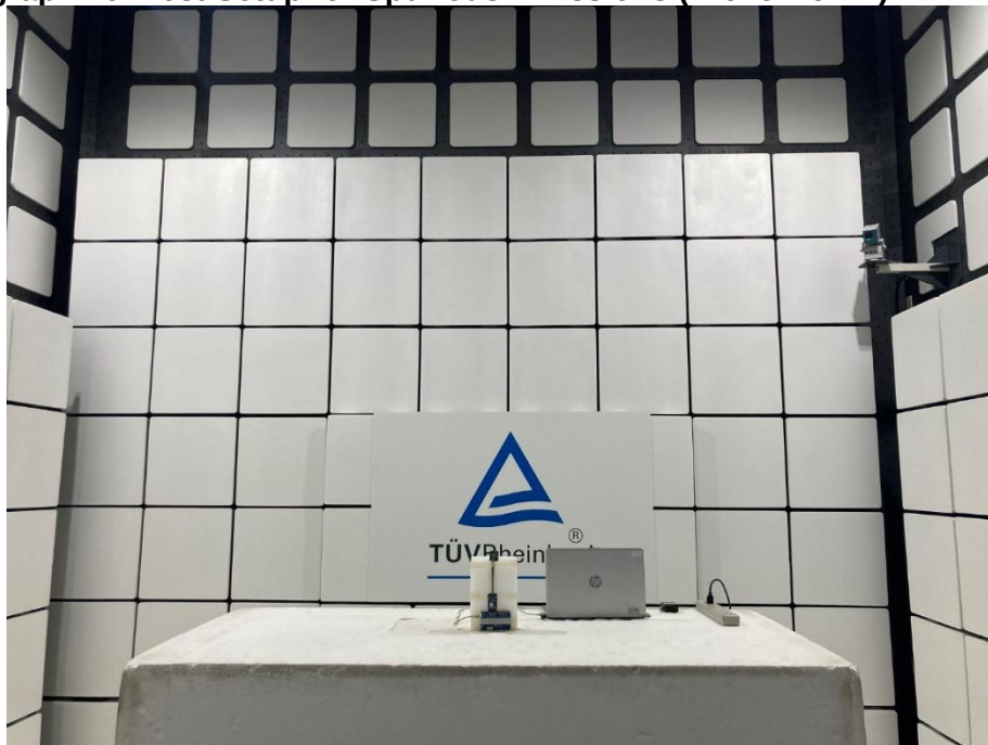
Photograph 10: Test Setup for Spurious Emissions (Front View 2)
