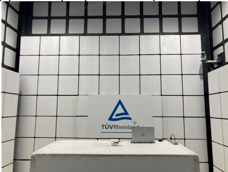
Photograph 2: Test Setup for Spurious Emissions (Front View 2)
