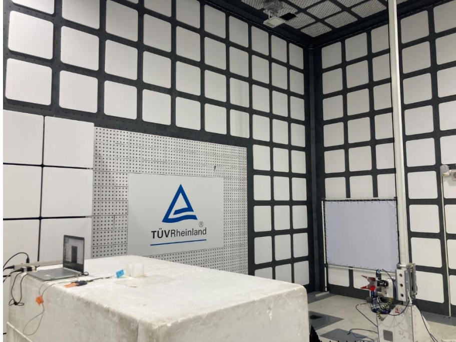
Photograph 5: Test Setup for Spurious Emissions (Back View 3)
