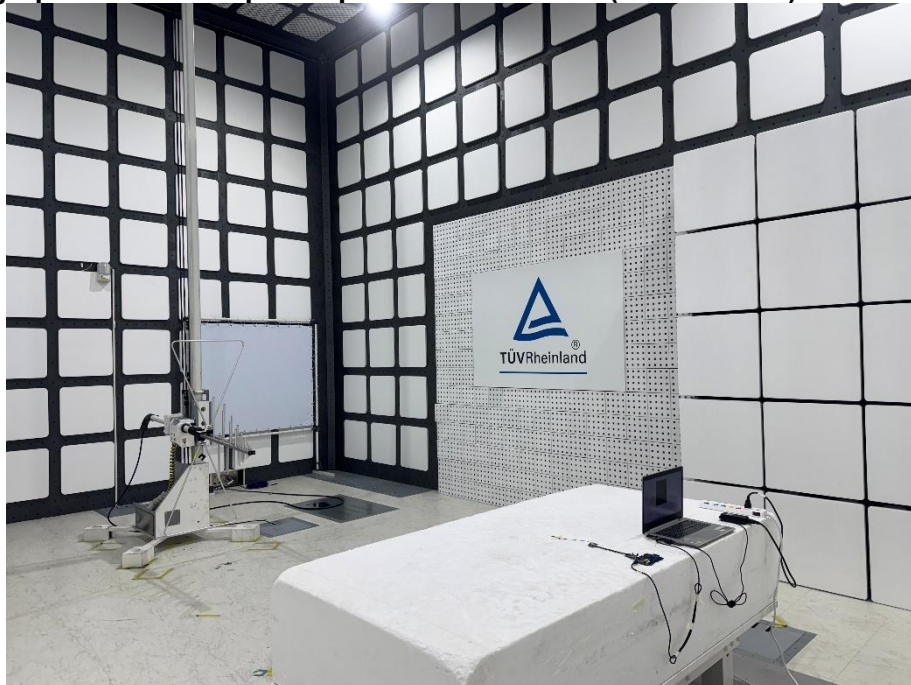
Photograph 8: Test Setup for Spurious Emissions (Back View 1)
