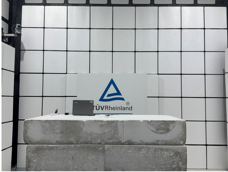
Photograph 8: Test Setup for Spurious Emissions (Back View 1)
