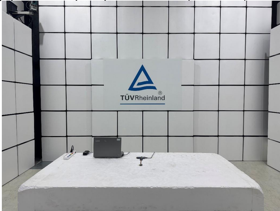
Photograph 2: Test Setup for Spurious Emissions (Front View 2)
