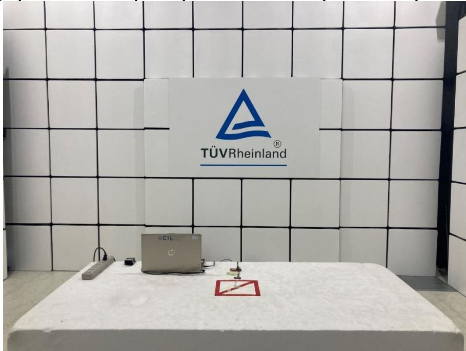
Photograph 43: Test Setup for Spurious Emissions (Front View 1)
