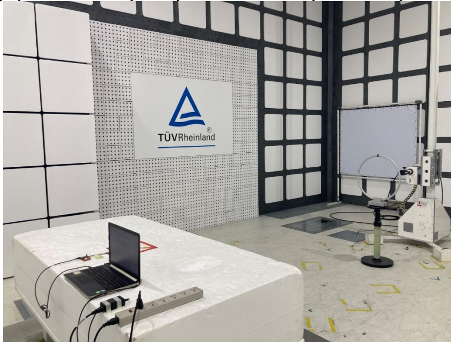
Photograph 46: Test Setup for Spurious Emissions (Back View 2)
