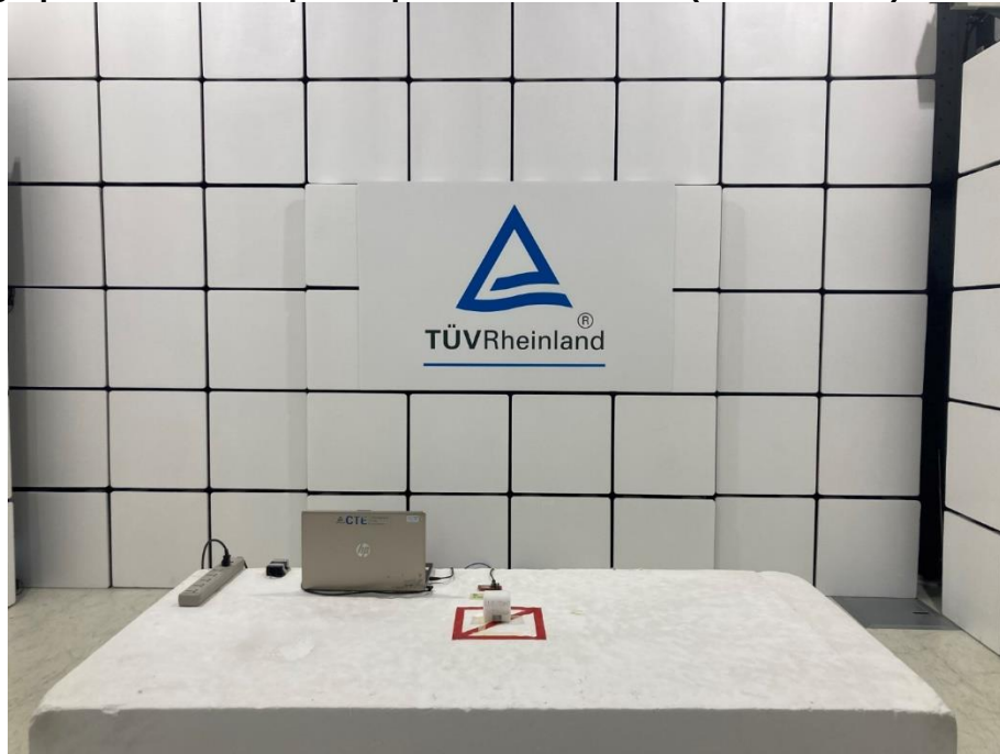
Photograph 37: Test Setup for Spurious Emissions (Front View 1)
