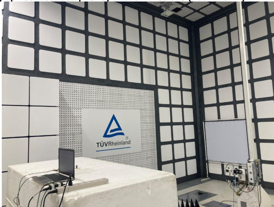
Photograph 30: Test Setup for Spurious Emissions (Back View 4)
