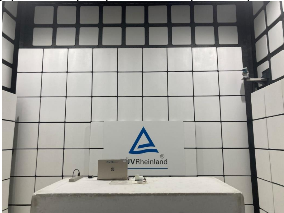
Photograph 2: Test Setup for Spurious Emissions (Front View 2)
