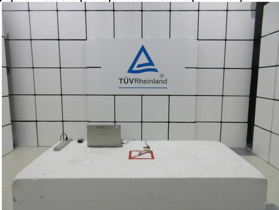
Photograph 52: Test Setup for Spurious Emissions (Front View)
