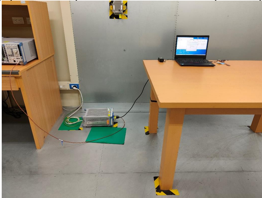
Photograph 13: Test Setup for Mains Conducted Emissions (Front View)
