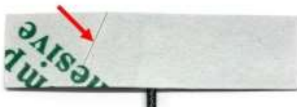
1. Find cut line on flex back side
