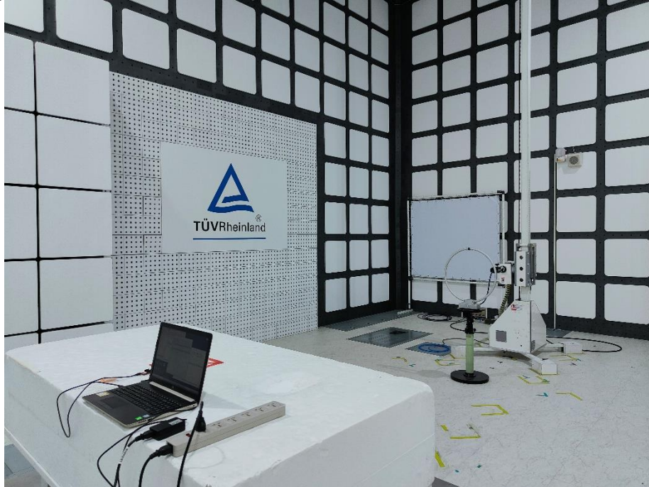
Photograph 9: Test Setup for Spurious Emissions (Back View 1, 2 nd Source)
