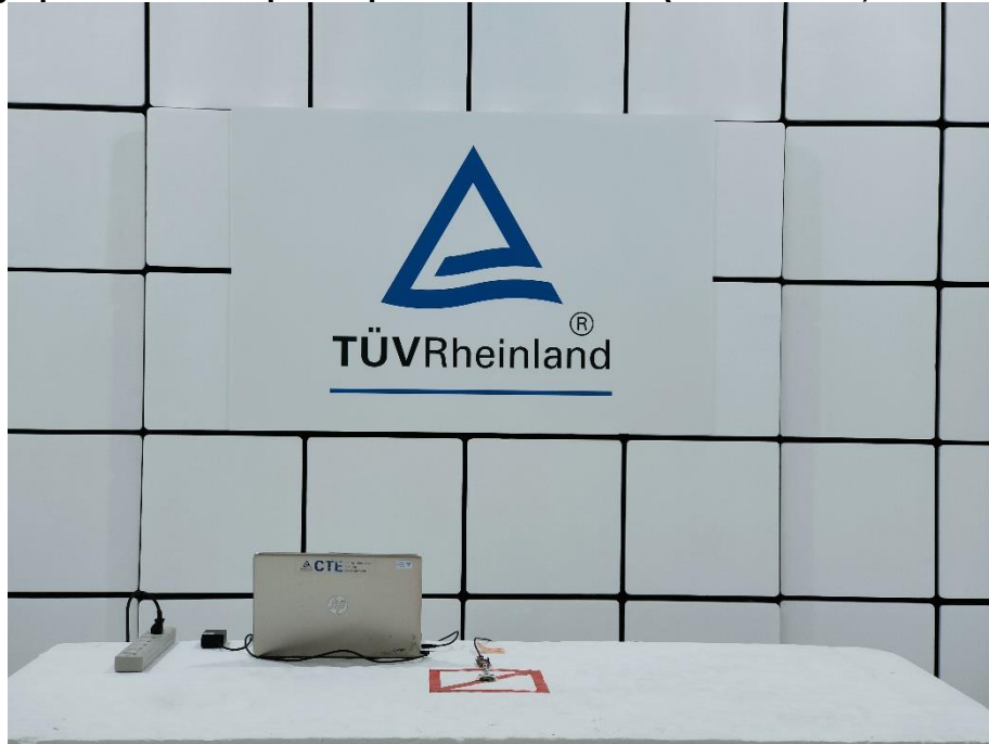
Photograph 1: Test Setup for Spurious Emissions (Front View 1, Main Source)
