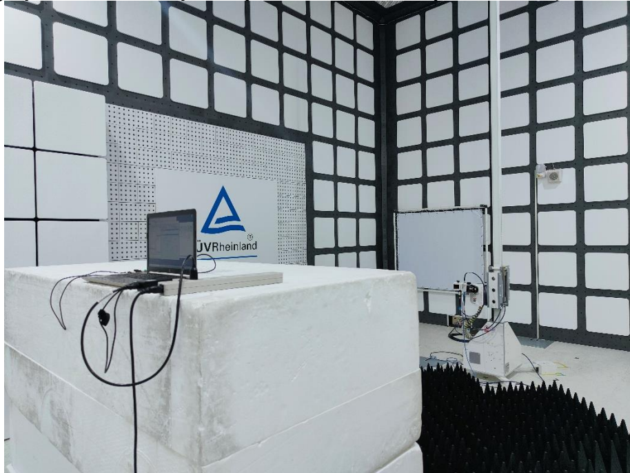
Photograph 12: Test Setup for Spurious Emissions (Back View 4, 2 nd Source)
