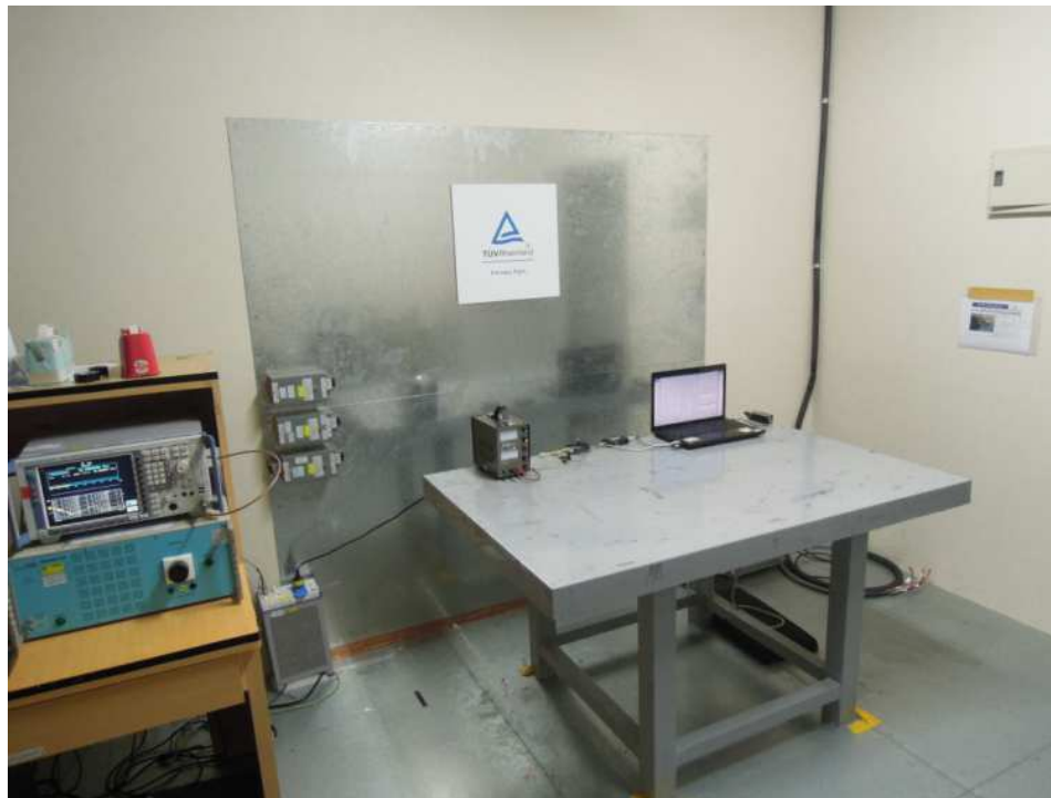
Photograph 21: Set-up for Mains Conducted testing (Front View)
