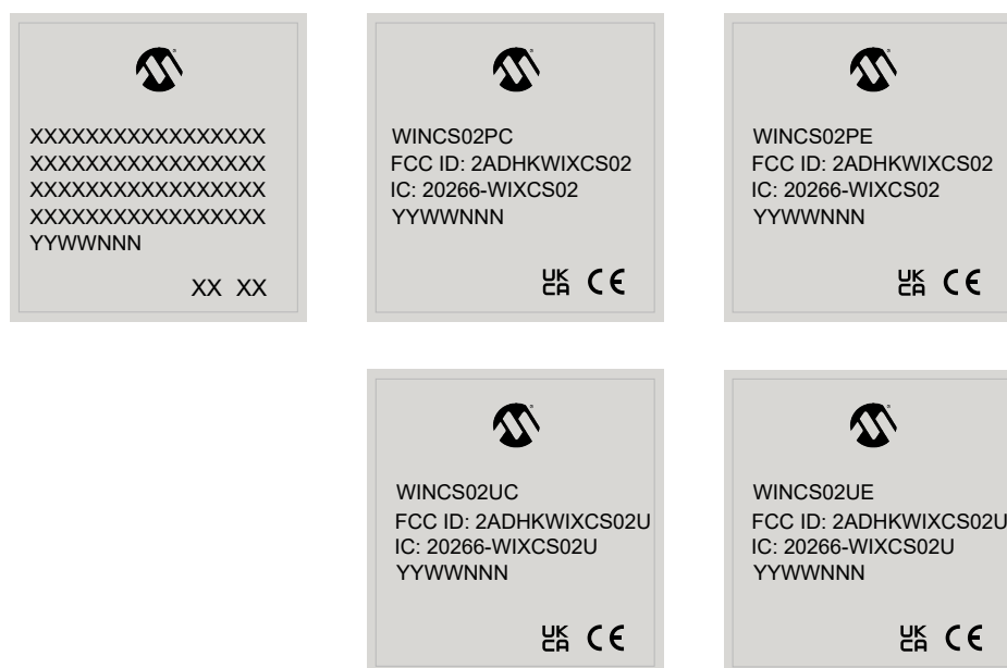
Figure 4-2. WINCS02 Module Packaging Marking
