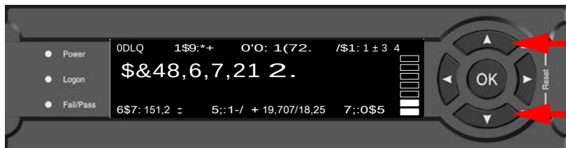
Figure 5-4: To reset the system
