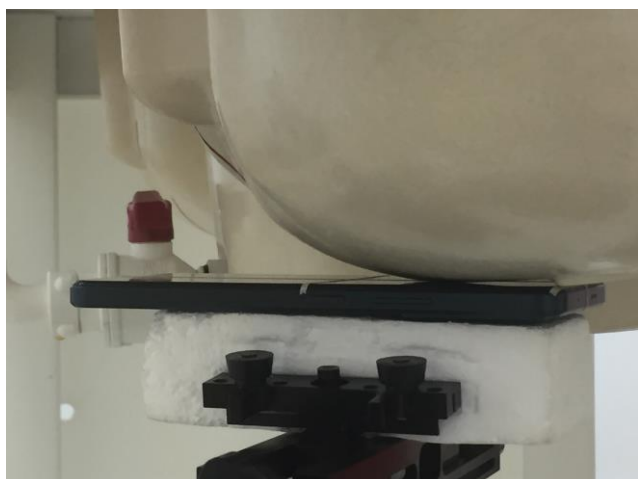
Left Cheek, Test Separation 0 mm
