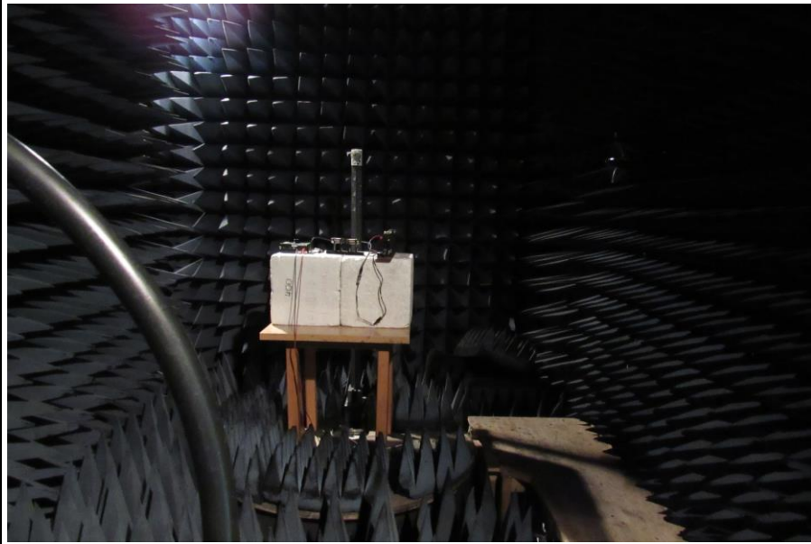
Setup radiated emission below 30 MHz
