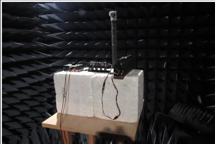
Setup radiated emission below 30 MHz Detail
