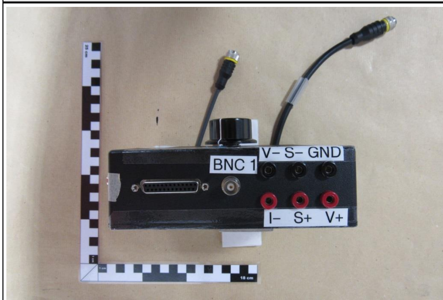
Test Box Connection Side 2
