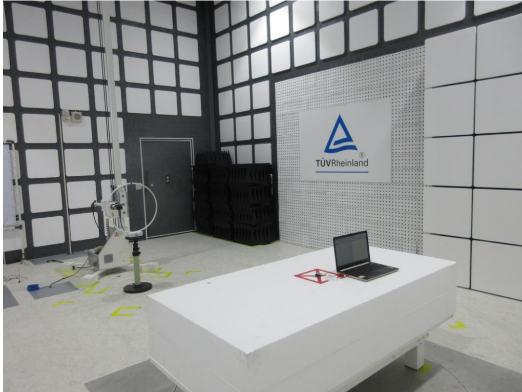
Photograph 5: Set-up for Spurious Emissions (Back View 3)
