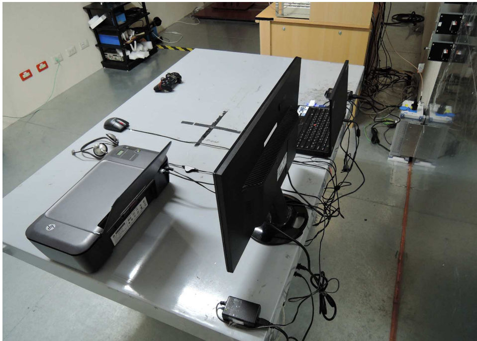
Photograph 5: Set-up for for Mains Conducted testing Back
