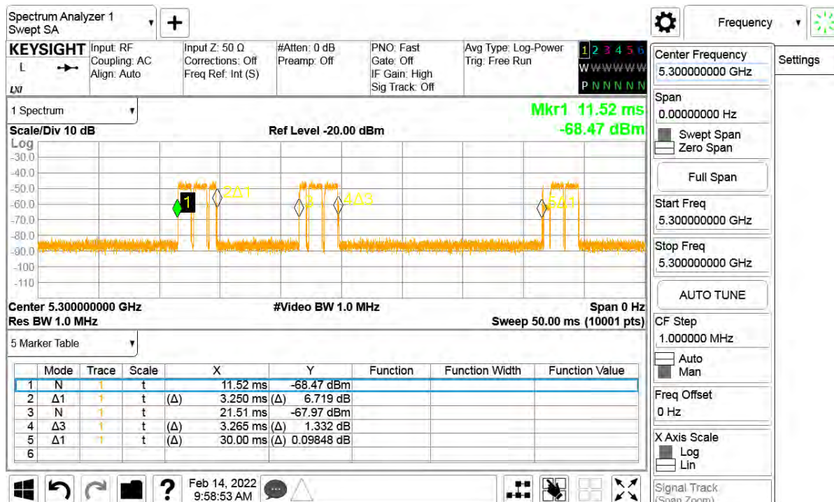
Plot of WLAN Traffic - 802.11ac (20 MHz), 5300 MHz
