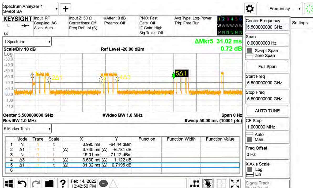
Plot of WLAN Traffic - 802.11ac (20 MHz), 5500 MHz
