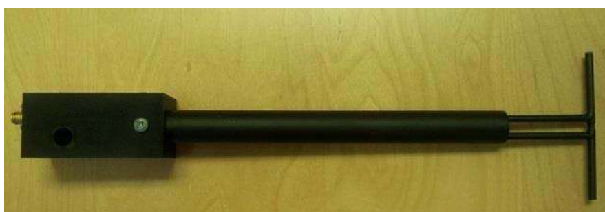
Figure 1 – MVG COMOSAR Validation Dipole
