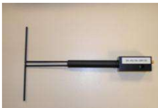
Figure 1 – MVG COMOSAR Validation Dipole
