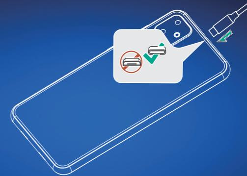
EN Insert USB cable and charge for 3 hours
