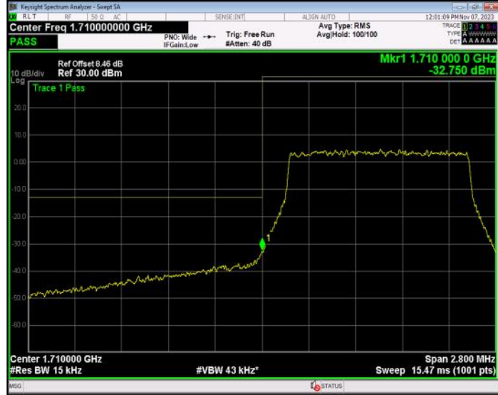
Band4 16QAM BW=1.4MHz Channel=20393 RB Size=6 Position=#0
