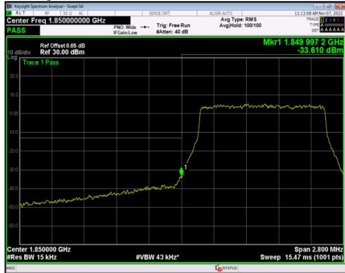
Band2 16QAM BW=1.4MHz Channel=19193 RB Size=6 Position=#0
