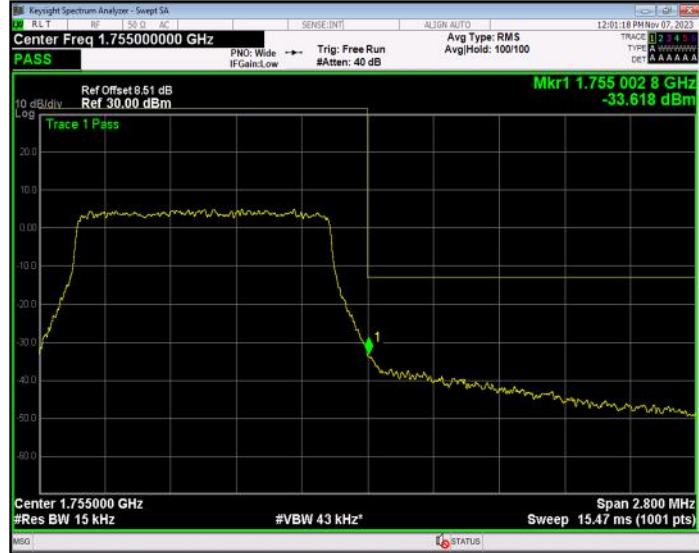
Band4 16QAM BW=10MHz Channel=20000 RB Size=50 Position=#0
