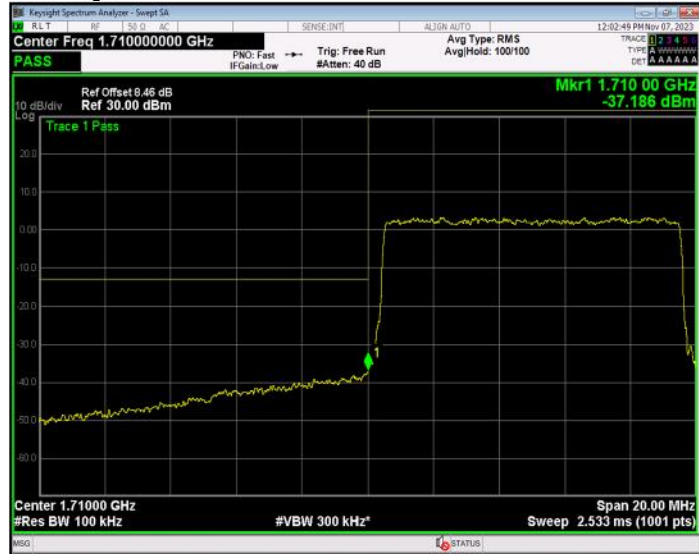
Band4 16QAM BW=10MHz Channel=20000 RB Size=50 Position=#0
