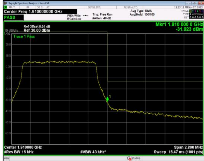
Band2 16QAM BW=10MHz Channel=18650 RB Size=50 Position=#0
