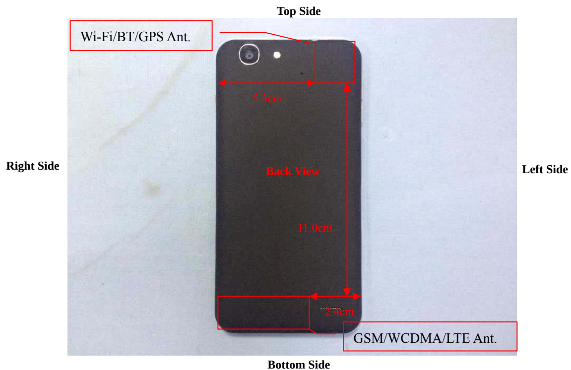
Block Diagram for EUT Antenna Position
