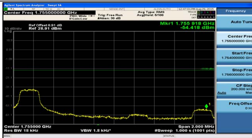
(Channel Bandwidth: 15 MHz)_HCH_QPSK_1RB#0
