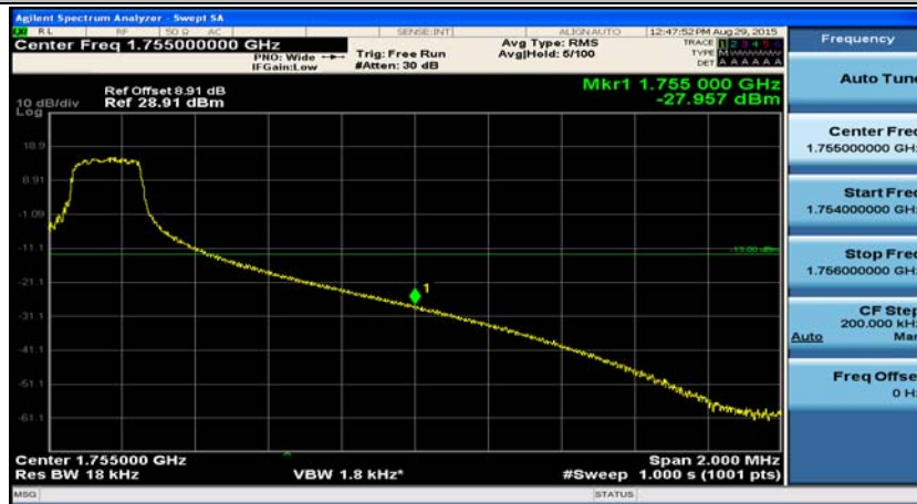
(Channel Bandwidth: 15 MHz)_HCH_16QAM_37RB#0
