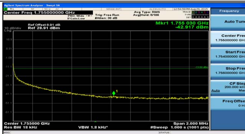
(Channel Bandwidth: 20 MHz)_HCH_16QAM_100RB#0
