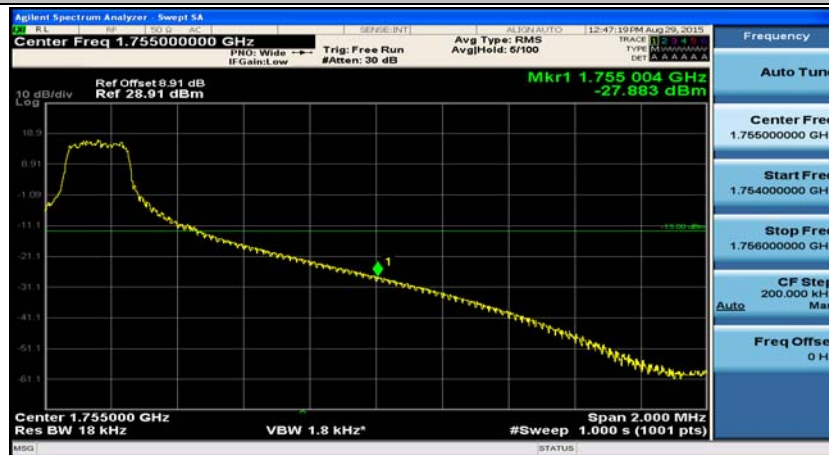
(Channel Bandwidth: 15 MHz)_HCH_QPSK_37RB#0
