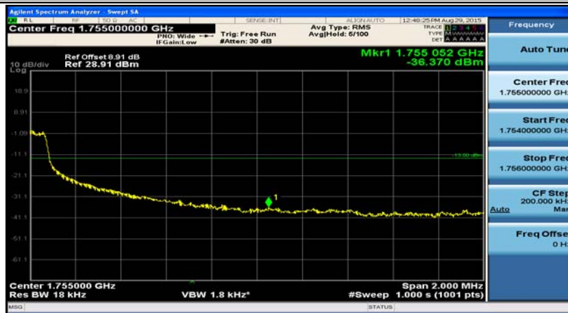
(Channel Bandwidth: 15 MHz)_HCH_QPSK_75RB#0
