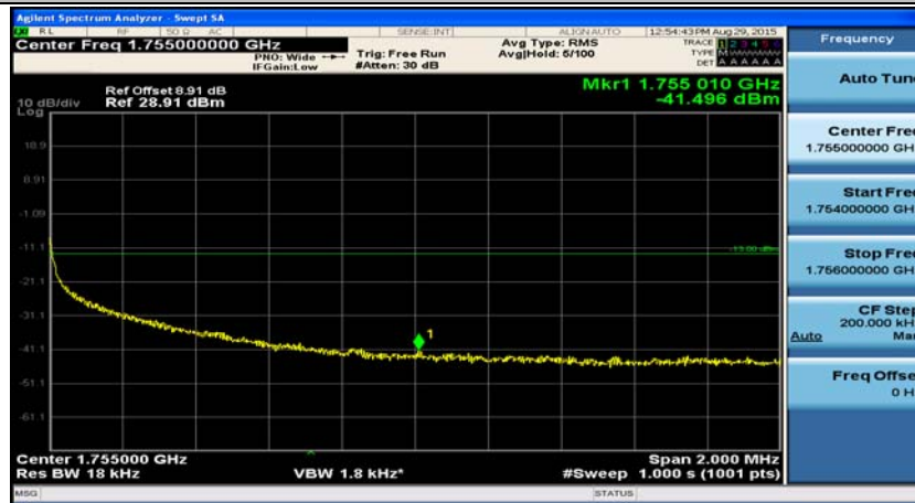
(Channel Bandwidth: 20 MHz)_HCH_QPSK_100RB#0
