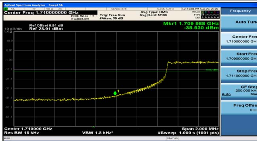
Channel Bandwidth: 10 MHz_LCH_QPSK_50RB#0
