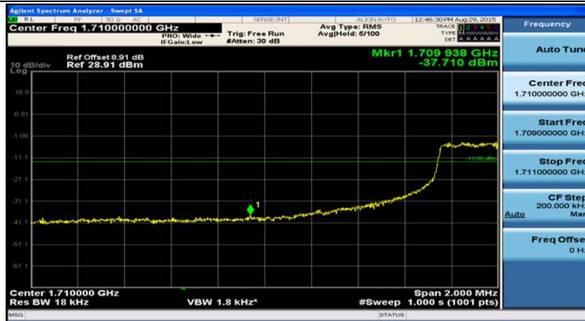
(Channel Bandwidth: 15 MHz)_LCH_QPSK_75RB#0
