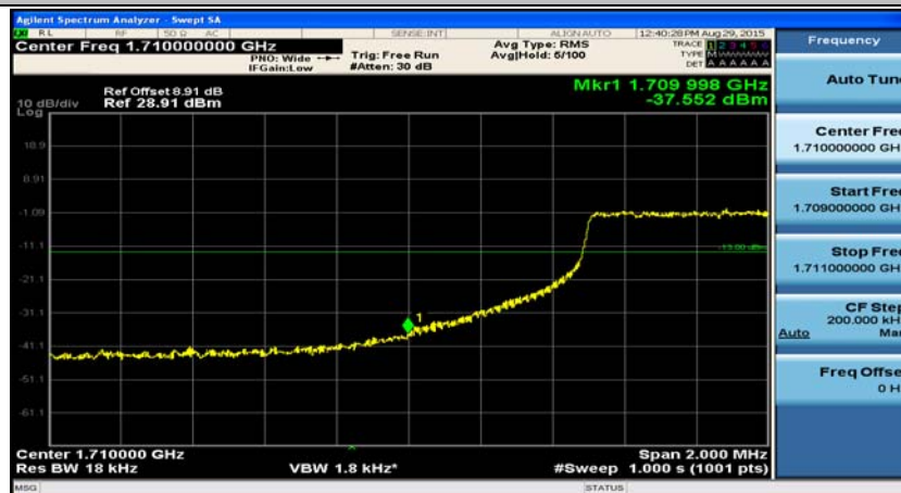
Channel Bandwidth: 10 MHz_LCH_16QAM_25RB#0
