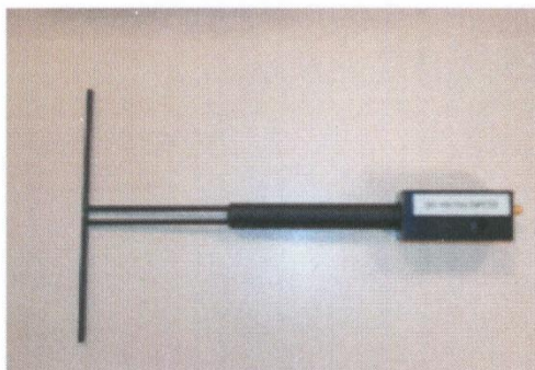
Figure 1 – Satimo COMOSAR Validation Dipole
