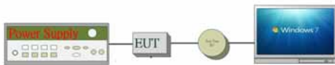
Fig. 2-1 Conducted (Antenna Port) Emission Configuration
