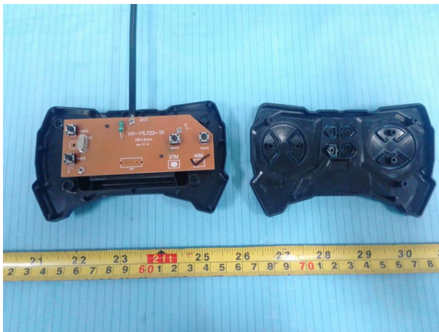
EUT – Cover off View 2
