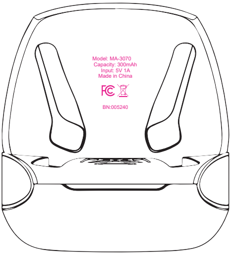
Laser engraved on the inside of the top cover 激光雕刻在充電盒蓋子的裏面
