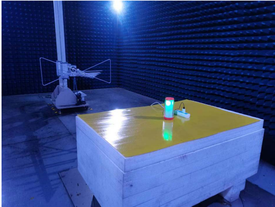
Photo of Radiated Emission Measurement Below 1GHz
