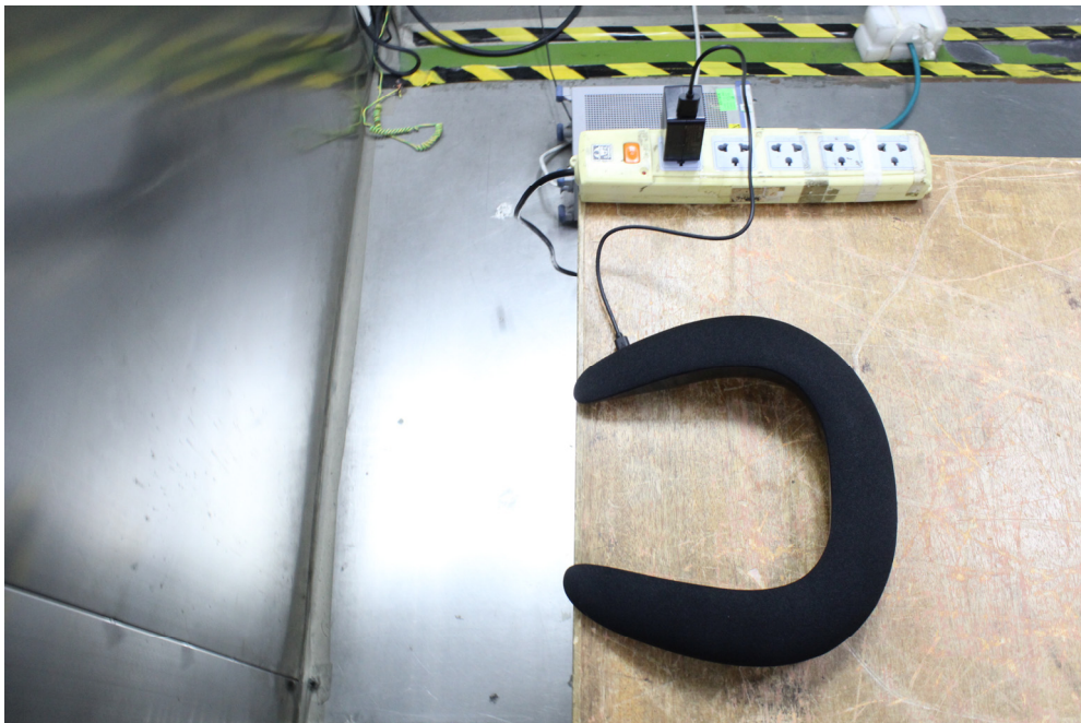
Conducted Emissions - Side View
