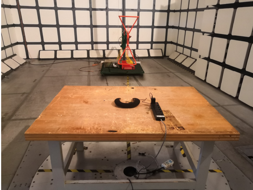
Radiated Emissions View (Below 1 GHz)
