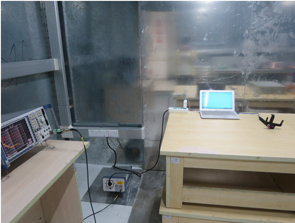
FCC RADIATED EMISSION TEST SETUP
