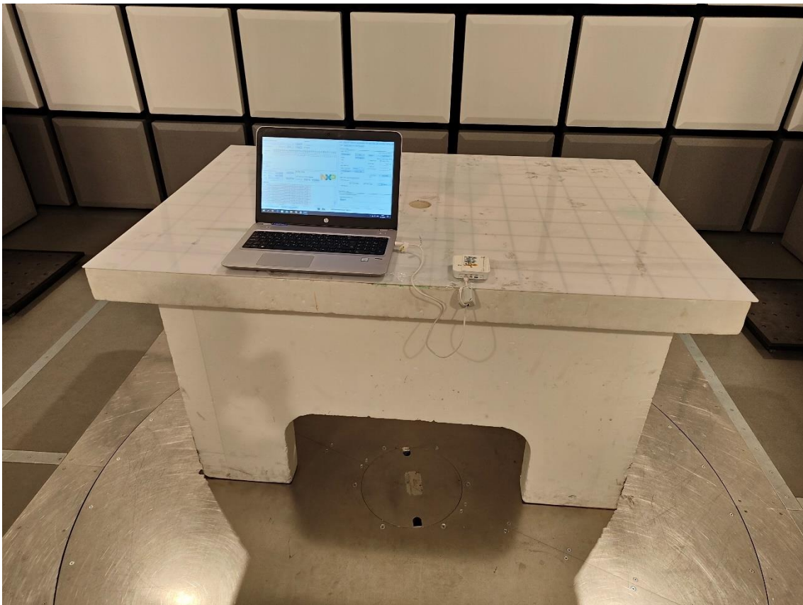
Figure 3: Radiated emission test till 1 GH
