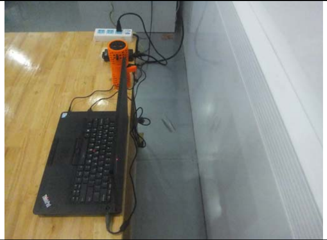
Conducted Emissions Test Setup Side View
