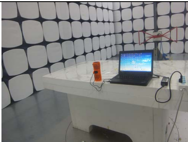
Conducted Emissions Test Setup Front View
