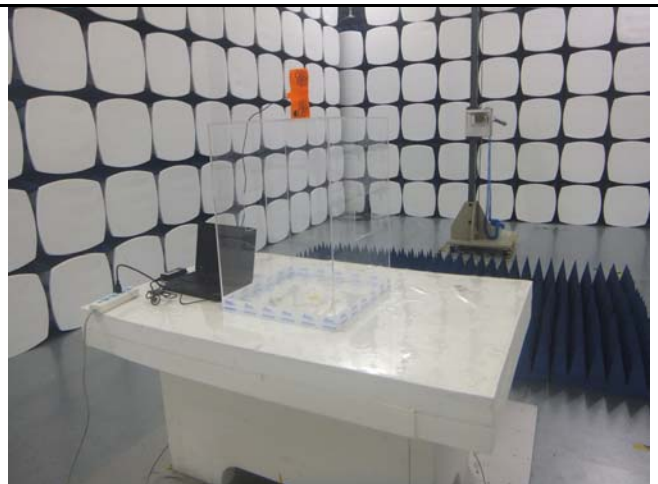
Radiated Spurious Emissions Test Setup Above 1GHz
