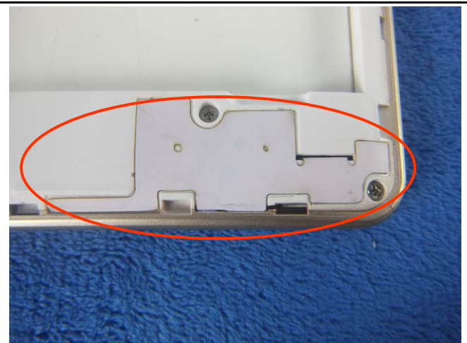
GSM/PCS/UMTS-FDD Antenna View
