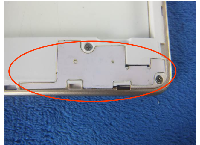
GSM/PCS/UMTS-FDD Antenna View
