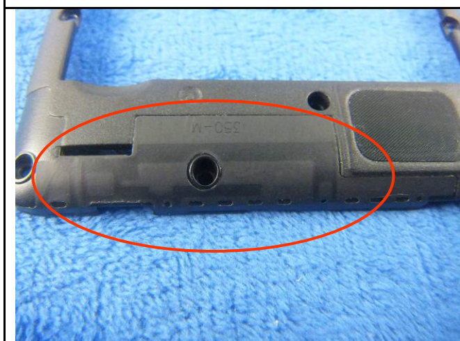
GSM/PCS/UMTS-FDD/LTE Antenna View
